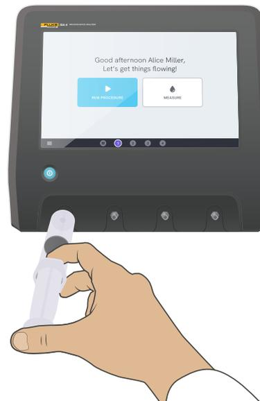
**Figure 24:** Draining a channel.
