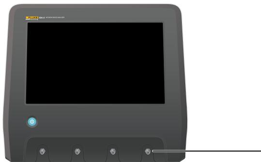
**Figure 8:** Reference height for pressure.
