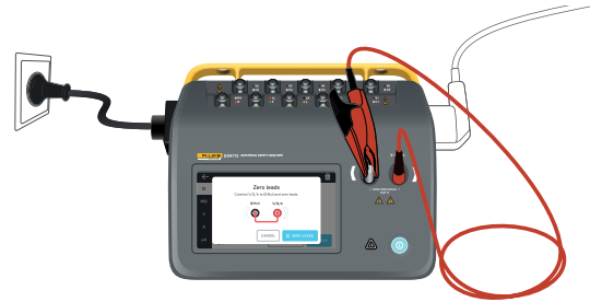
Figure 9: Setup for zeroing at protective earth resistance measurements, using one test lead and the null post adapter.
