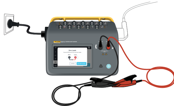
Figure 10: Setup for zeroing at point to point resistance measurements, using two test leads.
